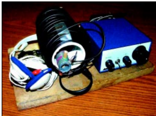
Success! Everything fits on a 1-square-foot tile on the kitchen floor. The key is mounted to the pine board, which protects the hardware against travel damage. A small tuner is (at the upper left) hidden under the rest of the station.
