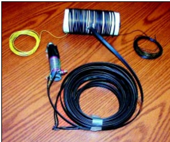
The Junk Box Shorty Forty—with the yellow and black dipole elements wound onto the loading coil—packed for transport. Note the twin lead connection to the middle, with two full turns between feed points. The 4:1 balun is visible as well.
